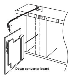
4 Insert the other end of the cable into the connector on the board itself.
