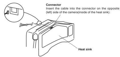
Remove the blank panel (right side of camera), then feed the cable (supplied with the board) through the rectangular opening under the top panel and insert it into the connector on the opposite side.
